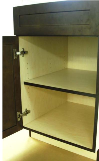
**Lastly adjust the door (s) if need be by tightening or loosening hinge screws. The screws that are not connected to either the carcass or door adjust the door left, right, front and back.**
