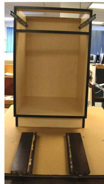
Detach A1 & B2 from A & I (sliders come off, using black clip attached to slider (Left side push up, Right side push down) and then pull drawer slides out until drawer is free)
